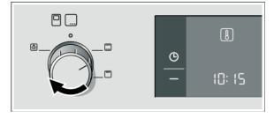
Set the temperature or grill setting using the temperature selector.
