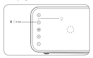
Press and hold the Bluetooth button for 2 seconds, and the light flashes blue.
