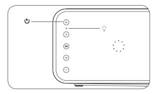
Press the power button to switch on, the light turns solid white.
